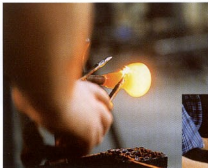
At first a small gather of glass is taken from the oven –
