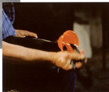
this will be blown, opened and spun into a rondel.
