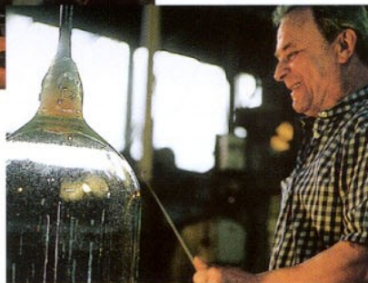
Top: The blowing of the molten glass takes place over a pit.
