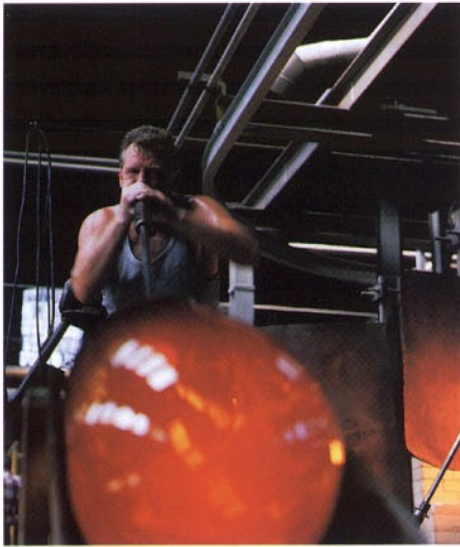
Above picture: The glass is blown into a ball-like form, cut open and flattened into a sheet.
