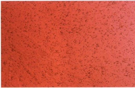
Small bubbles (known as seeds) are one of the most important characteristics
