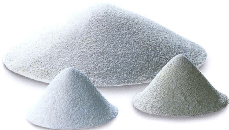
The basic ingredients of glass are quartz sand, soda and lime.
